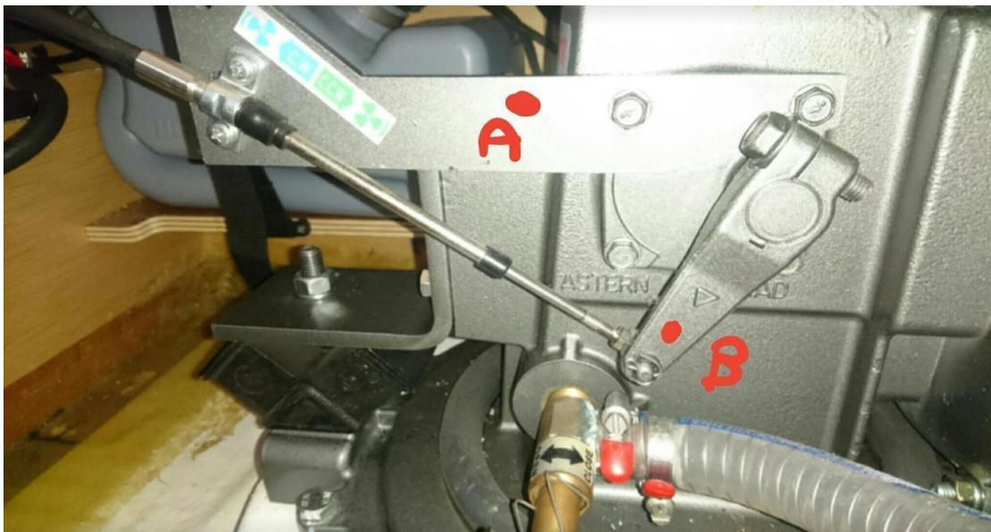
2. Arrangement for Volvo engine. The image should represent the neutral position. Holes "C" and "B" would appear to be already present. Creating a new hole in "A". Placing the gear forward would bring the two holes "C" and "A" to overlap. A new hole about in "D" could be considered to make the leaded cable work easily in the transitions from neutral to reverse.
